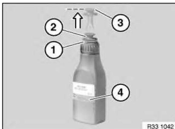
Tear off and remove the lead seal (1) between the thread on the bottle and the filler neck stopper.
